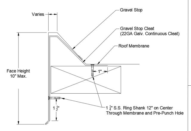
**Material Type** Finish: Color: 24 GA 22 GA **Roof Material:** .032" AL **Membrane Thickness:** .040" AL Substrate: .050" AL Wood Masonry
